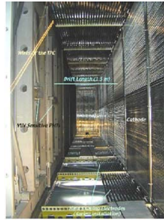
Fig. 17. Icarus T600 detector during installation
