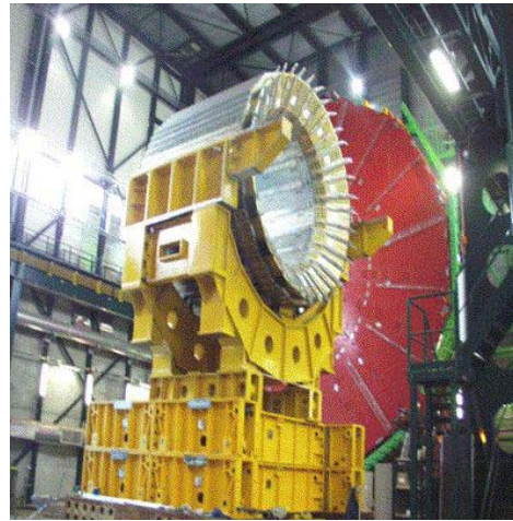
Fig. 33. The hadronic barrel calorimeter of CMS in the assembly hall
