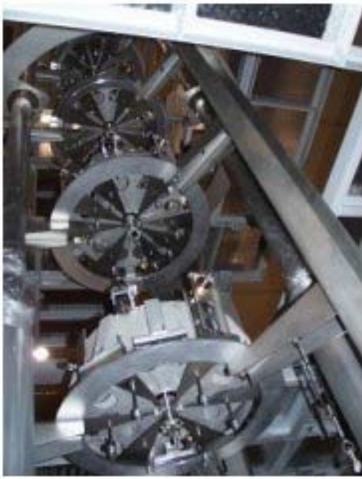
Fig. 3. A Virgo mirror suspension tower (height about 10 m)
