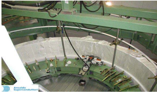
Fig. 28. CMS solenoid: winding of first longitudinal section
